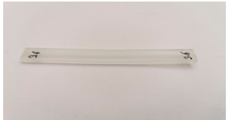
Sample exhibiting the highest plastic flexural deformation following three-point bending of Sample D specimens.
