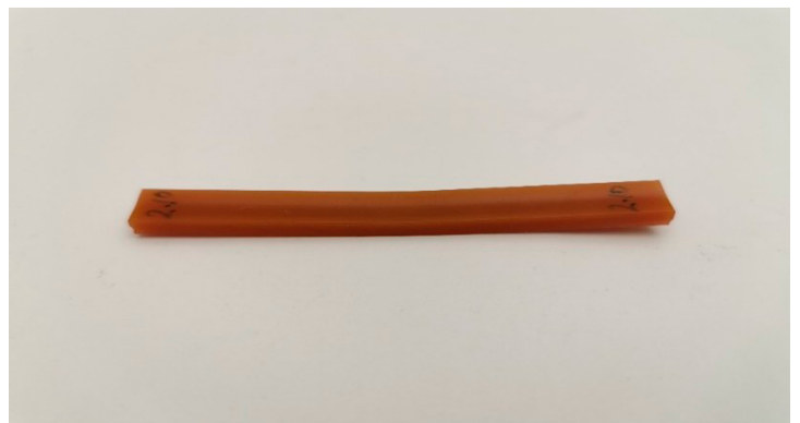
Sample exhibiting the highest plastic flexural deformation following three-point bending of Sample B specimens.
