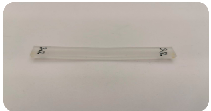
Sample exhibiting the highest plastic flexural deformation following three-point bending of Sample E specimens.
