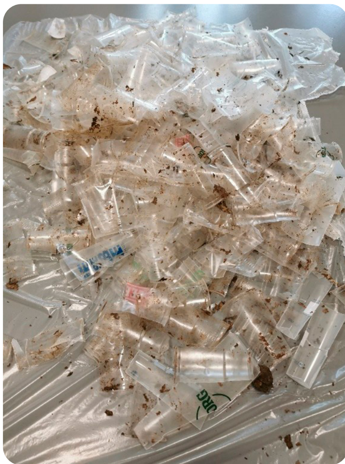
Figure 1: Recovered Aarhus River polypropylene fraction (Sample A) prior to cleaning and mechanical processing, showing visible dirt and adhered residues.
