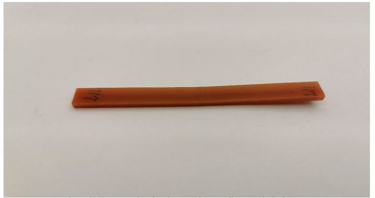
Sample exhibiting the highest plastic flexural deformation following three-point bending of Sample C specimens.
