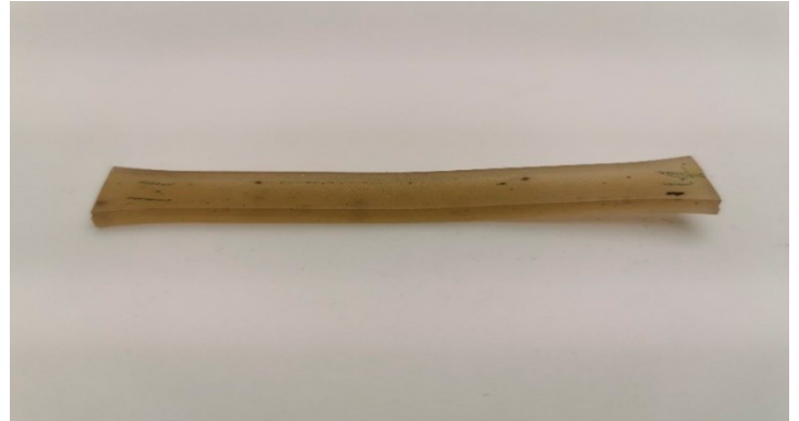
Sample exhibiting the highest plastic flexural deformation following three-point bending of Sample A specimens.
